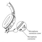
1) Microphone installation Push the cover upward to open the microphone connector to plug in microphone.
