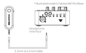
Note: In order to avoid signal interference, when your audio interface is connected to smartphone via Bluetooth, you need to add a 3.5mm extension cable in between the transmitter and the guidio interface
